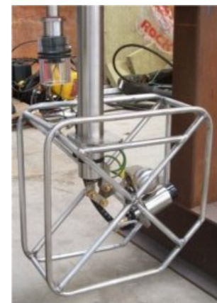
Gas detector with video camera and light
